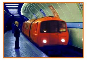
The circular route is almost 6.5 miles (10.5 km) long and extends both north and south of the River Clyde. The tracks have the unusual gauge of 4 foot (1,219 mm). The system was modernised between 1977 and 1980 including the provision of new rolling stock. New signalling was installed in 1996.
