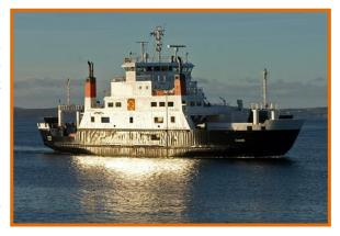
ship's design is unique as she has bow and stern ramps, allowing drive-through operation, and also a port side ramp, allowing side-loading on the Clyde in the winter months. The Schottel azi-pod propulsion system is used by the ship and this incorporates rotating pods protruding beneath the hull, with two propellers on each.
